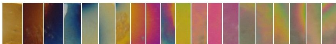
Figure 3. Sections of surfaces of the anodising nanograin Grade 2 titanium discs, with voltage changing from left to right from 10 to 200 V in 10 V increments
