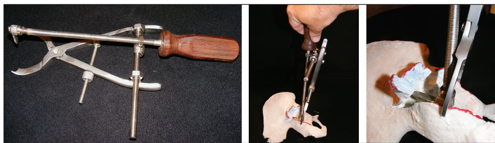
Figure 14. The use of the instrument required for the lateral bending of the block on a model
