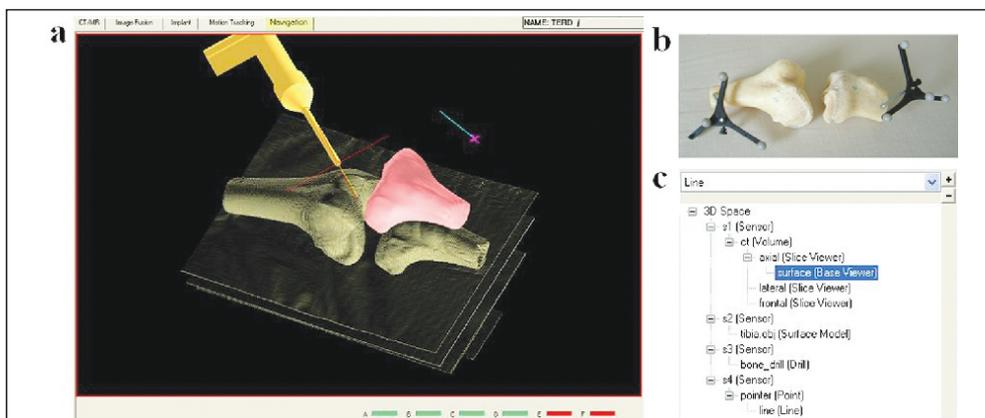
*Figure 4.* Framework application. Illustration of a cadaver experiments based on movement recording of tibia relative to reference coordinate space set on the femur. The movable model of tibia is created from the isosurface rendered model by suitable surface reconstruction algorithm (a). The sensors are attached to the bone parts (b) and the topological relationships are planned by the navigation tree; the experiment needs two more sensors to track movements of the pointer and drill (c)
