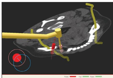
*Figure 6.* The virtual scene of handpiece navigation in computerized implantology. It prepares the placement of dental implant into the lower jaw. Targeting aid can be seen in the left bottom corner. The same visualization can be used during intraoperative navigated drilling of jaw bone or template preparation for drill-guiding holes
