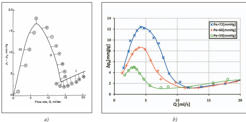
Figure 10. Pressure differences along a collapsible tube as a function of the volumetric flow rate. a) the curve measured by Conrad<sup>6</sup>; b) the results of our measurement
