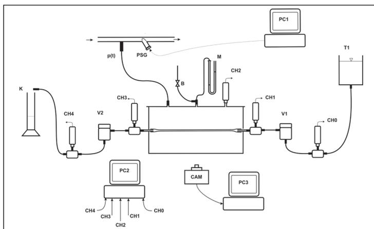
Figure 3. Sketch of the measuring equipment for unsteady reservoir pressure
