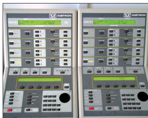
Figure 1. The consols of the Instron 8874 biomechanical material testing machine
