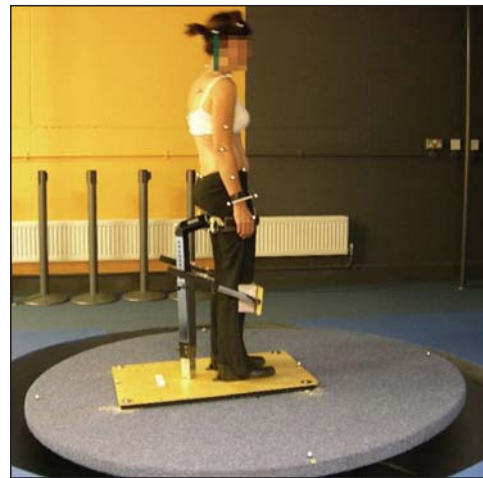
Figure 2. The upper part of a Targeted Training equipment is mounted on the CAREN platform which was programmed to replicate the default rocking movement normally provided by a rocker base. Responses of hip and lumbar flexion/extension were recorded and compared to a condition in which the body was rotated around an axis joining the two hip joint centres
