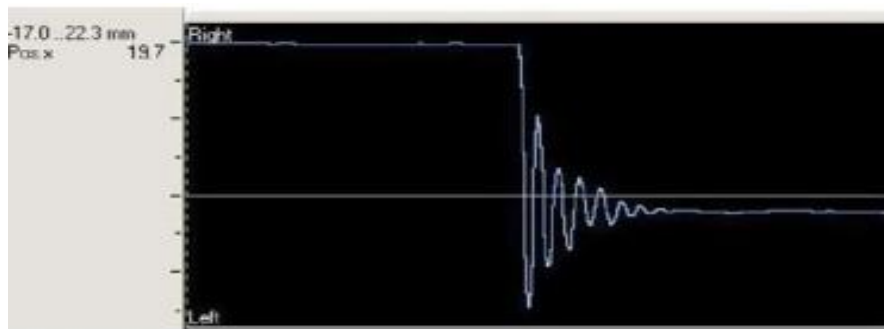
Figure 4. Damping curve_1. Lateral displacement of the measuring plate calculated from the spatial coordinates of the markers. The coordinate x is parallel to the direction of provocation and shows a damping curve.
