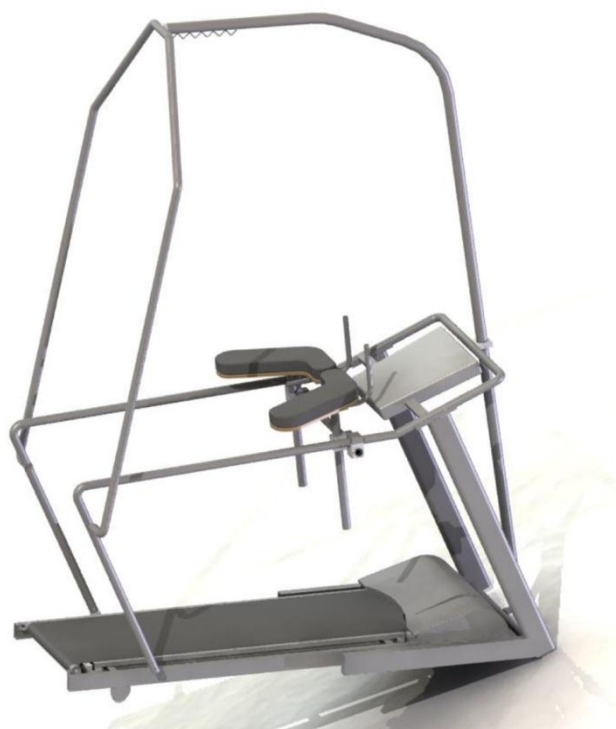
Figure 10. 3D view of force transducer treadmill
