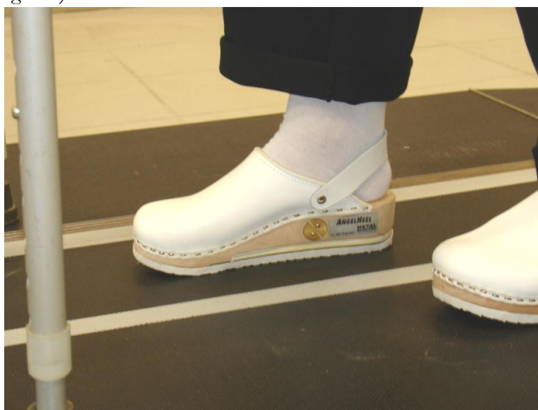
Figure 2 Force transducer shoes on the scale platform
